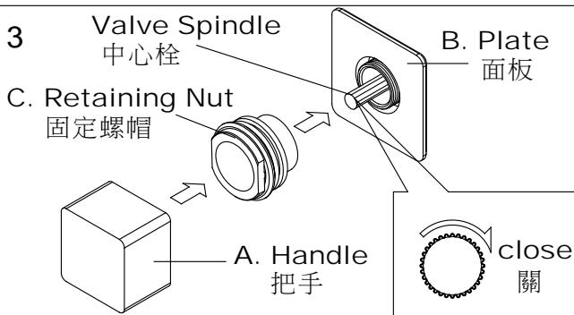
3. Turn the Valve clockwise to closed position before install Handle. Fix the Plate against the wall with Retaining Nut, and then press Handle onto Valve Spindle till hears the "CLICK" sound to finish the installation.
