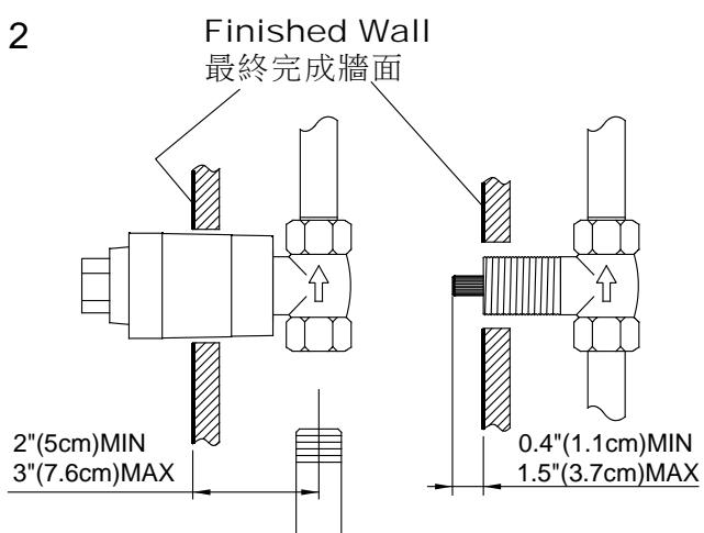
1. Use Sleeve to protect the cartridge and thread before installation.
