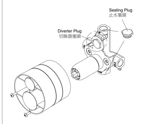
\* The Sealing Plug should be used as installing Concealed Mixer Valve (W/O Diverter Version).
