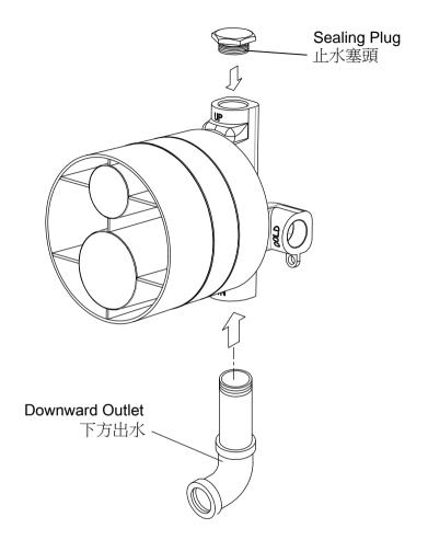
\*Installing the Downward Outlet, and screw the Sealing Plug to upward outlet of valve body.
