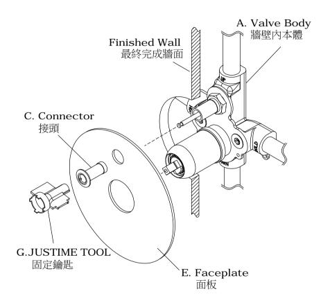
\* Install the **Faceplate** to flush with the wall,and tighten the **Connector** with **JUSTIME TOOL**.
