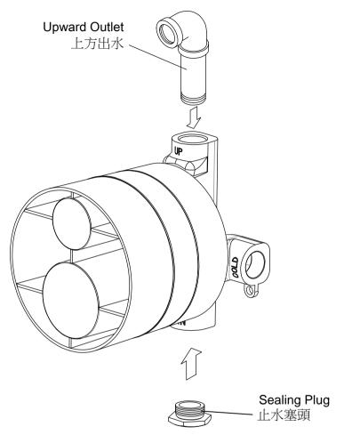
\* Installing the Upward Outlet, and screw the Sealing Plug to downward outlet of valve body.
