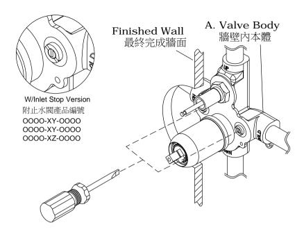
\* Operate the Inlet Stop Valve with Slotted Screwdriver.
