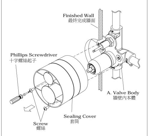
\* Disassemble the **Screws** with **Phillips Screwdriver** to remove the **Sealing Cover**.
