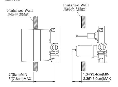
\* Connect hot and cold supply pipes to the valve body and meantime install outlet water ways, and keep the distance between 2"(5cm) minmum and 3"(7.6cm) maximum from the finished wall to the valve body; or keep the distance be 1.34"(3.4cm) to 2.36"(6.0cm) between top of cartridge and Finished Wall for necessary conditions.
