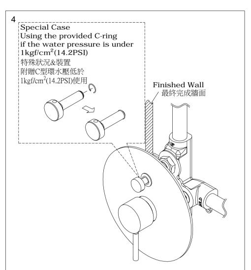
\* If the water pressure is too high, please adjust the water flow with Handle to operate the diverter.
