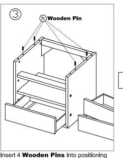
holes on top edge of **Table Cabin** for locate **Table Deck** as shown in figure #3. Take out the drawers from Table Cabin for next step.
