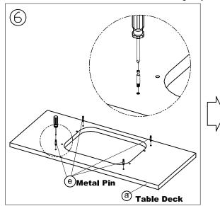
Screw and secure 4 Metal Pins firmly into backside of Table Deck as shown in figure #6.
