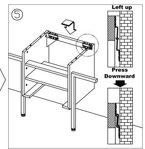
Position the Table Cabin close to the wall, lift up and locate the table's back-brackets on the Wall Brackets, then press Table Cabin downward to lock both **Brackets** together as shown in figure #5.
