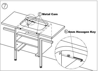
Press and join the two pieces of Table Deck and Table Cabin together with Wooden Pins, then insert 4 Metal Cams into holes inside of Table Cabin, rotate Metal Cams clockwise and tighten them with Metal Pin by attached **Hexagon Key**.
