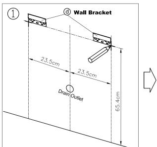
Mark two vertical lines both sides 23.5cm (9.25") from the center of drain outlet, and meantime, locate the Wall Bracket on show positions, then use the Wall Bracket as a template and mark the drilling holes position on the wall with the small holes of Wall Bracket as shown in figure #1. The big holes on Wall Bracket are for sleeve anchor fixing only.
