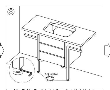
Level the Table Deck by twisting adjustable table feet.
