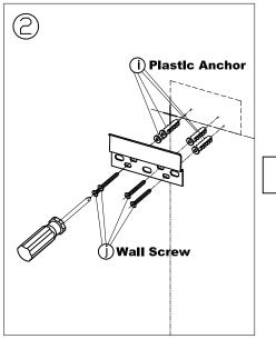
Fix Wall Brackets on certain position and tighten Wall Screws.
