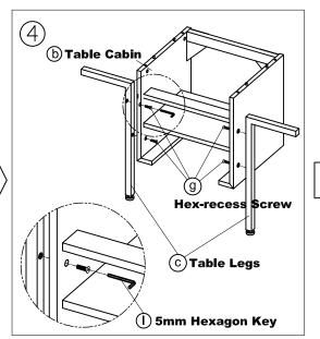
Assembling the Table Legs both side on the Table Cabin with Hex-recess Screws by 5mm Hexagon Key.
